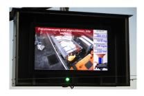
Monitoring of the loading process conveniently from the driver's cab by means of an installed screen
